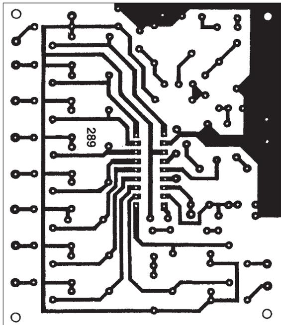
Fig. 11. Full-size Multi-purpose L.E.D. Driver foil master.
