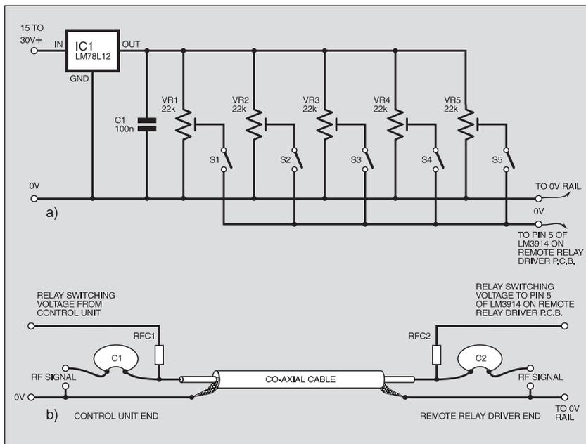
Fig. 8. Control Unit and applying switching voltages via an r.f. signal cable. (a) circuit diagram and (b) cable interlink details.
