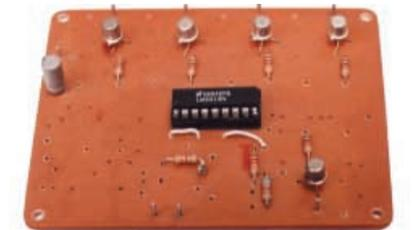
Remote Relay Driver circuit board. See Fig.7 for circuit diagram and Fig.10f for board details. It is possible to control up to 10 relays, using the control board of Fig.9.
