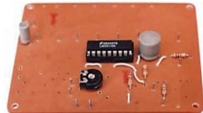
Bargraph display with "warning" flasher. Sensitivity adjustable from 1.25V upwards. See Fig.4 for circuit and Fig.10c for board details.
