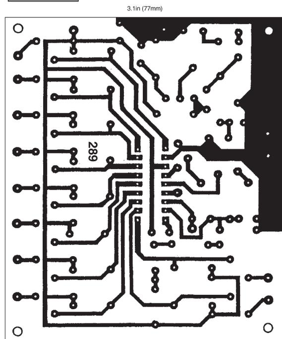
Fig. 11. Full-size Multi-purpose L.E.D. Driver foil master.
