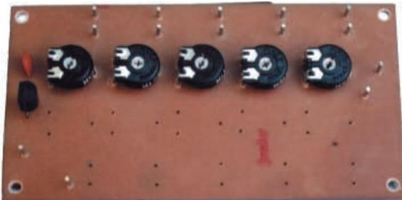
Relay Control board (for 5 relays).
