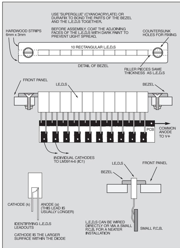
Fig.3a. Assembly details for making the l.e.d. bargraph.
